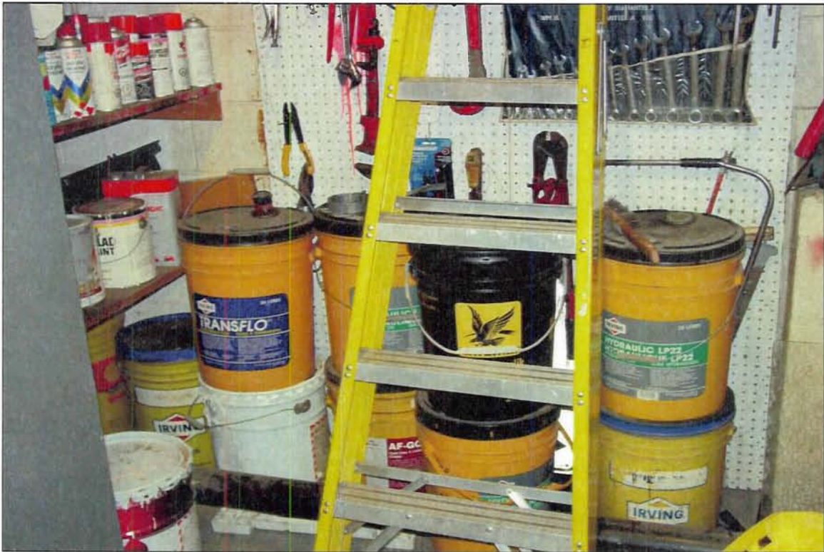
Photo 10 - Paints And Oils Stored In Unventilated Room
