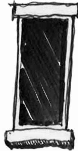
No full glazed infill windows
