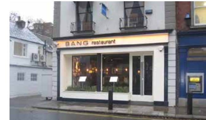
Effective use of a colour scheme integrated with fascia signage. Quality pin-mounted letters
